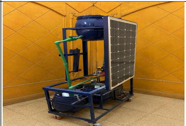
This solar-powered water lifting system includes a water pump with a single-phase electric motor.
